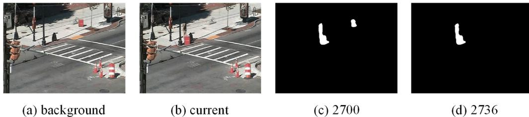
Figure 4: Intermittent object detection on abandonedbox sequence. Background object leaves the background region and ghost appears in the original position. When counters reach the own critical value, pixels in the ghost position are immediately updated to the background samples.
